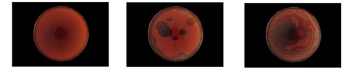
Sample of waves created in Petri dish during BZ reaction
